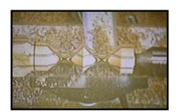
The block was turned to a cylinder and using a template the design was transferred to the piece. Large coves were turned with a spindle gouge on both sides of the centre. Carlyn worked alternately on each cove, taking the same cut on each so as to keep them uniform in shape and size. The coves were deepened until the laminations near the centre of the block became visible. At this point the coves were sanded through the grits and the hole to take the corkscrew was drilled in the central portion.
